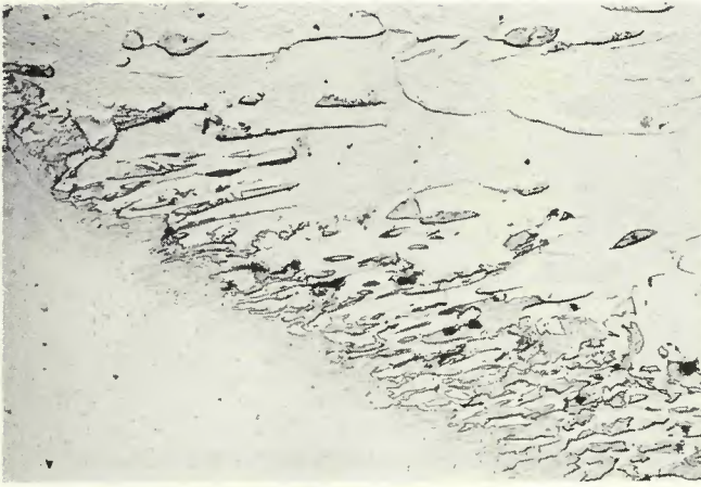
Fig. 5 — Carbon replica of interface structure in stress relieved joint. X2000, reduced 25%
