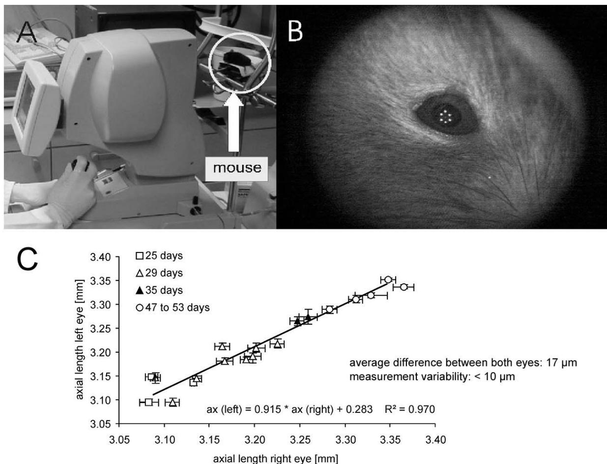
**Figure 4.** Optical low coherence interferometry in mouse eyes. (A) The slightly anesthetized mouse, positioned on an adjustable platform which is attached to the chinrest of the AC Master, is encircled. B. Close-up view used to adjust the eye in the measurement beam. The first Purkinje images of 6 infrared LEDs, built into the device, are used to align the eye. (C) Quality of the axial length data obtained with the AC Master - a plot of left versus right eyes (replotted after 24).
