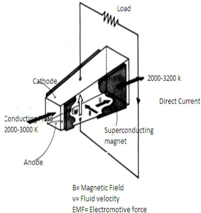
Fig.1. Principle of operation of MHD Generator
