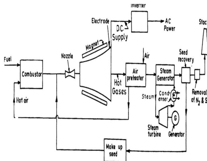
Fig. 2. A Schematic Diagram For open Cycle MHD
