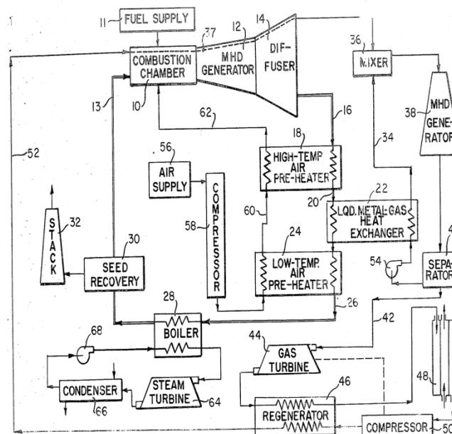
Fig. 3. A Schematic Diagram For open Cycle MHD
