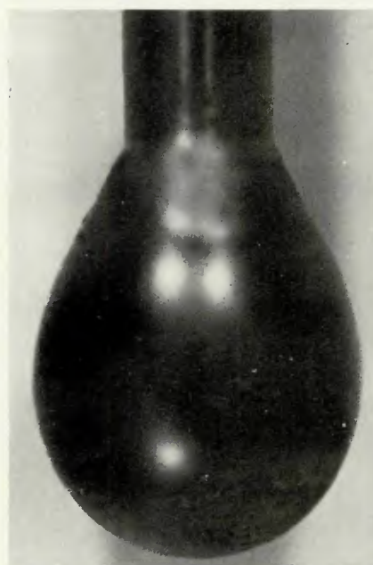
Fig. 6—Typical pendant drop used for determination of the liquid-vapor boundary tension of a metal. \times 9.2
