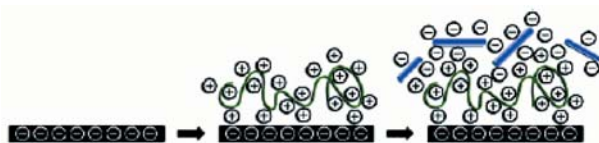
Figure 8. Schematic representation of the build-up of electrostatically adsorbed multilayered films. The polyelectrolyte, cationic poly(allylamine hydrochloride), is shown by the curved line and colloidal cellulose nanocrystals are represented by straight rods; counterions have been omitted for clarity
