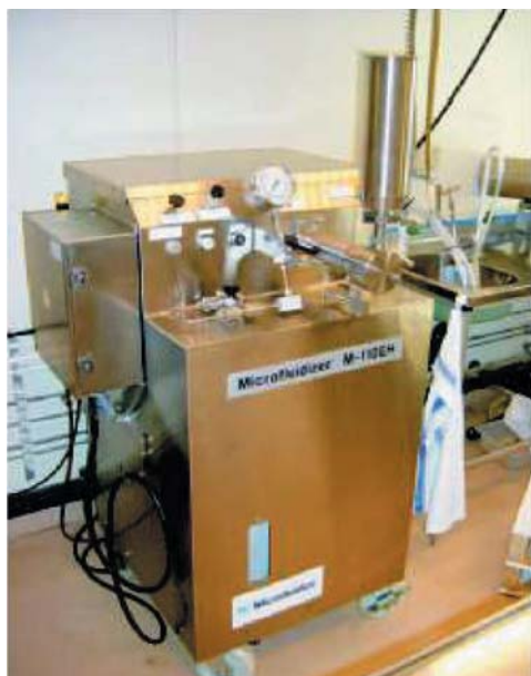
Figure 5. Homogenizer (Microfluidizer) used for the production of microfibrillated cellulose
