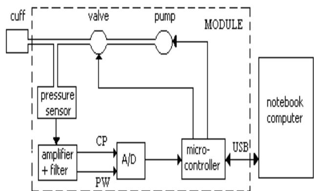
Fig. 2. Block diagram of the system's module.
