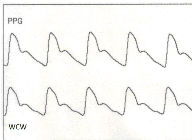
Fig. 4. Waveforms obtained from a finger photoplethysmograph (PPG) and waveforms from a wrist cuff (WCW).
