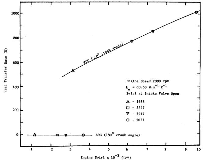
Fig. 5 Effect of Swirl on Heat Transfer Rate
