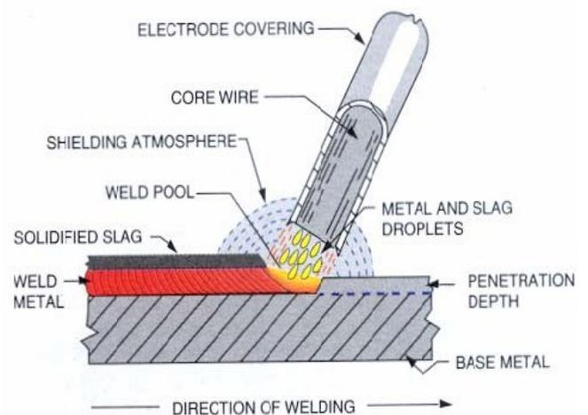
Fig.1.1 Shielded Metal Arc Welding Process (Genculu, 2011)
