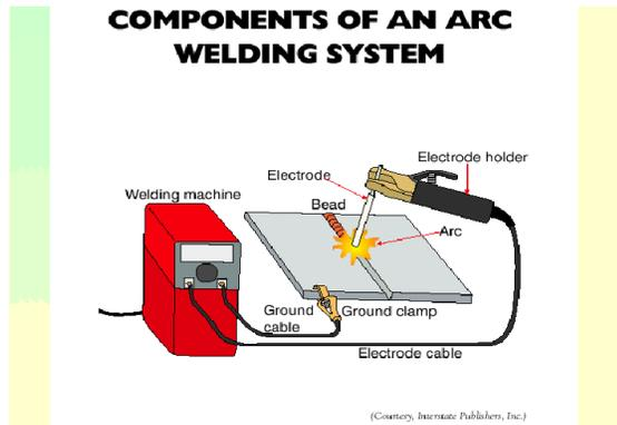
Fig.1.2 Set up Shielded Metal Arc Welding process
